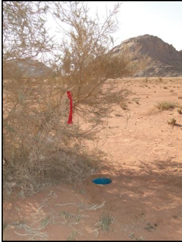
FIGURE 3. A pit-fall trap with a sign to facilitate location of the trap. (Photographed by Adel A. Ibrahim).
